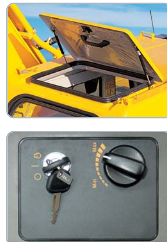
1 Wide, Comfortable Operating Space 2 Steel Cover Sunroof 3 Dial Type Engine Speed Switch and Key Switch
