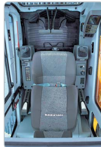
1 Wide, Comfortable Operating Space 2 Steel Cover Sunroof 3 Dial Type Engine Speed Switch and Key Switch
