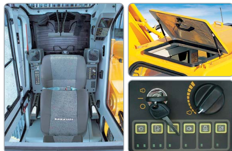
1 2 3 1 Wide, Comfortable Operating Space 2 Steel Cover Sunroof 3 Dial Type Engine Speed Switch and Key Switch
