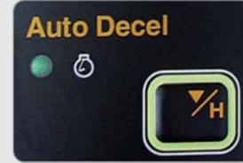
When remote-control valves are in neutral position more than 4 seconds, CPU controller instructs the accel actuator to reduce engine speed to 1200rpm. This decreases fuel consumption and reduces cab noise levels.
