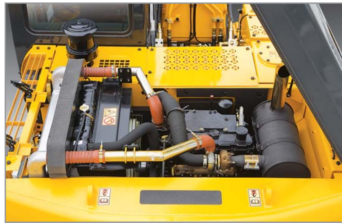
Easy to maintain engine components The cooling and preheating system are provided for optimum and immediate operation, guaranteeing longer life for the engine and hydraulic components. Servicing of the engine and hydraulics is considerably simplified due to total accessibility.
