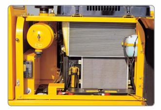
**Side Cover with Left & Right Swing Open Type**Easy access to vital components gives unrestricted view of
