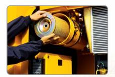
Centralized Electric Control Box and Easy Change Air Cleaner Assembly
