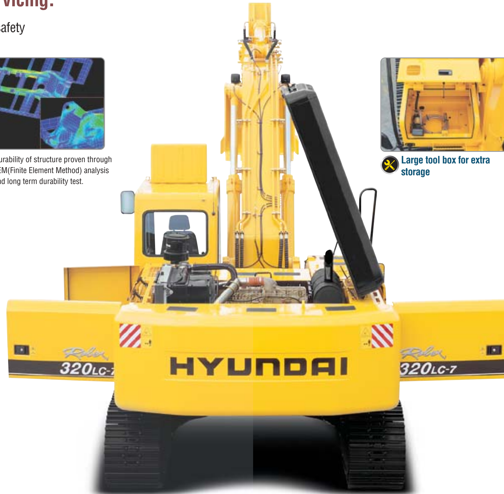
Side Cover with Left & Right Swing Open Type Easy access to vital components gives unrestricted view of component allows easy maintenance and repair.
