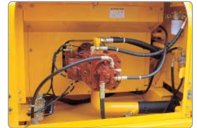
Highly efficient Hydraulic Pump Pump output and Hydraulic tank capacity have been increased. A pilot pump has been installed resulting in improved control sensitivity.
