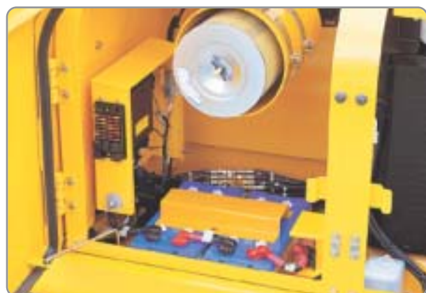
Centralized Electric Control Box and Easy Change Air Cleaner Assembly Electric control box and Air cleaner are centralized in one or the same compartment for easy service.
