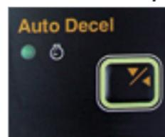
When remote-control valves are in neutral position more than 4 seconds, CPU controller instructs the accel actuator to reduce engine speed to 1000rpm. This decreases fuel consumption and reduces cab noise levels.
