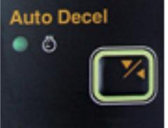
When remote-control valves are in neutral position more than 4 seconds, CPU controller instructs the accel actuator to reduce engine speed to 1000rpm. This decreases fuel consumption and reduces cab noise levels.
