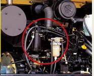
minimize the risk of fuel breakdown, high capacity fuel filter and transparent water separator are applied for durability.
