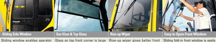
to communicate outside and air to enough to give better visibility view to operator. circulate without having to open while sun visor protects operator main door.
